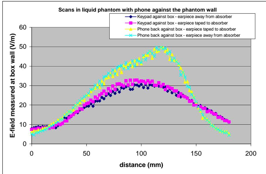
Figure 6: SAR scans inside the liquid-filled phantom along the mid-line of the Nokia 3210 phone (placed against the outside of the box). The earpiece is at left and phone is centred at the point 90mm on the distance axis. The SAR is higher when the back of the phone is placed against the absorber and is slightly influenced by whether the earpiece is also against an absorber.
