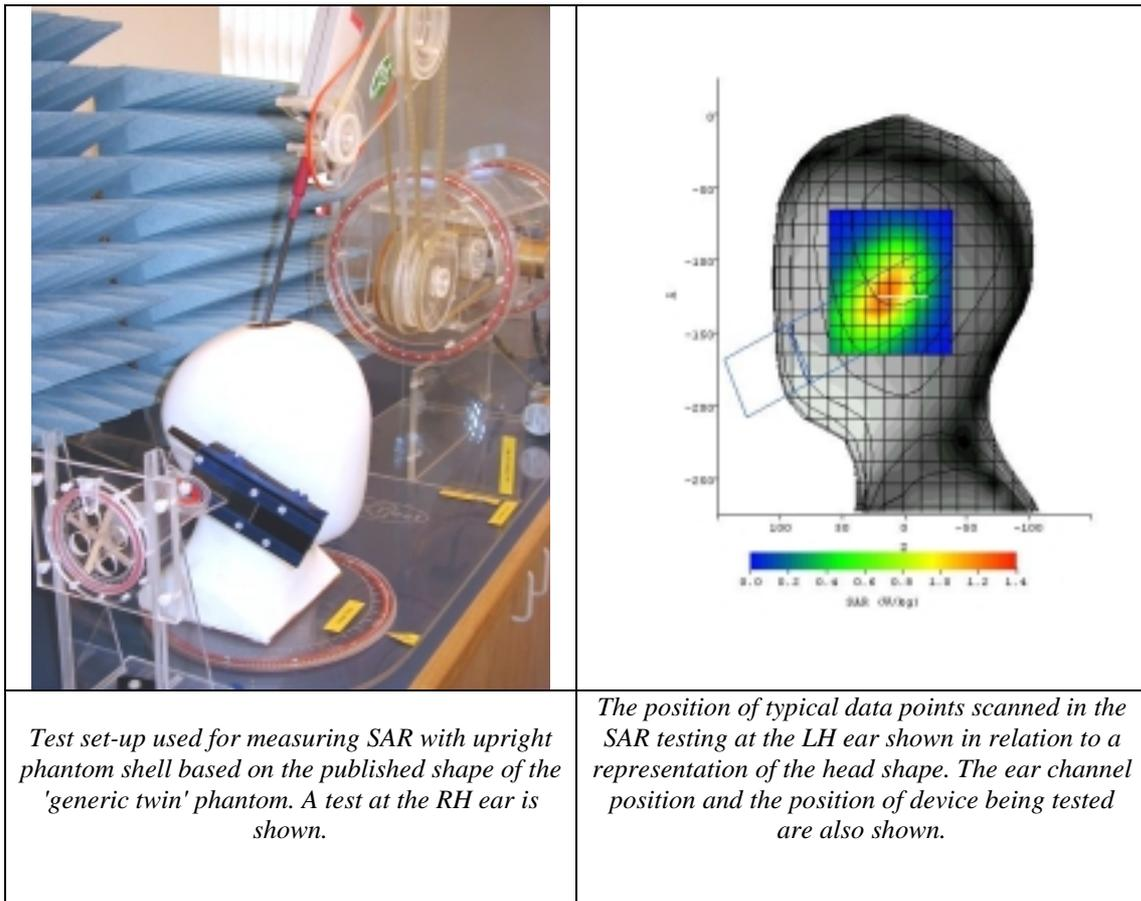
Figure 7. Test set-up used for measuring SAR .
