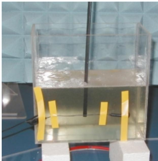
*Figure 3: Showing the earpiece cable taped horizontally to a box-shaped phantom with the probe articulated within the box.*
